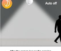
After the person leaves the sensing range for 50-60 seconds, it automatically turn off 4.
